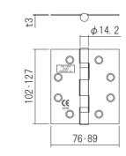
The number of hinges required Door height (mm) Hinges Quantity Below 1523 1524~2285 3 2286~3048 4
